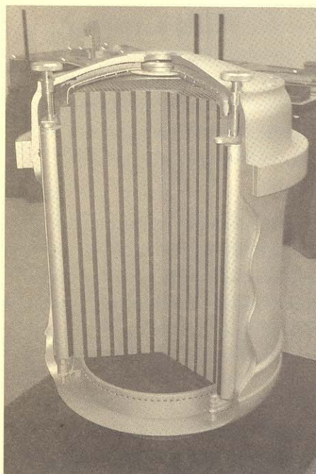
Cut-away scale model of a Project Rover nuclear rocket engine at the NTS History Center, showing the nuclear fuel rods stacked through the center of the engine cylinder, surrounded by turnable neutron absorption and reflection control rods. In the inverted testing mode, hydrogen gas was fed into the bottom of the engine, and exited as high temperature rocket propulsion gases through an inverted rocket nozzle placed on top of the engine.
